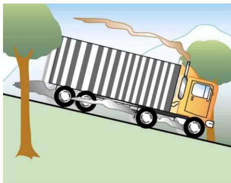
Figure 14.4: The smoking brakes on this truck are a visible evidence of the mechanical equivalent of heat.
