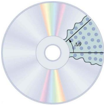
Figure 6.1: All points on a CD travel in circular arcs. The pits along a line from the center to the edge all move through the same angle \Delta\vartheta in a time \Delta t .
