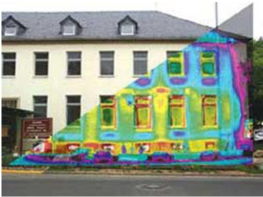
Figure 14.16: A thermograph of part of a building shows temperature variations, indicating where heat transfer to the outside is most severe. Windows are a major region of heat transfer to the outside of homes. (credit: U.S. Army)
