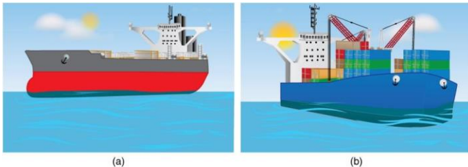
Figure 11.17: An unloaded ship (a) floats higher in the water than a loaded ship (b).
